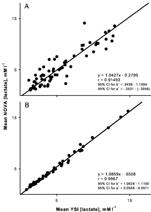
**Figure 3** Ordinary least products regression analysis of the relation between lactate concentrations determined by the Lactate Plus portable analyzer and the YSI bench top analyzer. (A) When separate samples for each analyzer were collected directly from finger. (B) When a common sample of blood was used by both analyzers. Regression equations and CIs for slope (B) and y-intercept (A) are presented.
