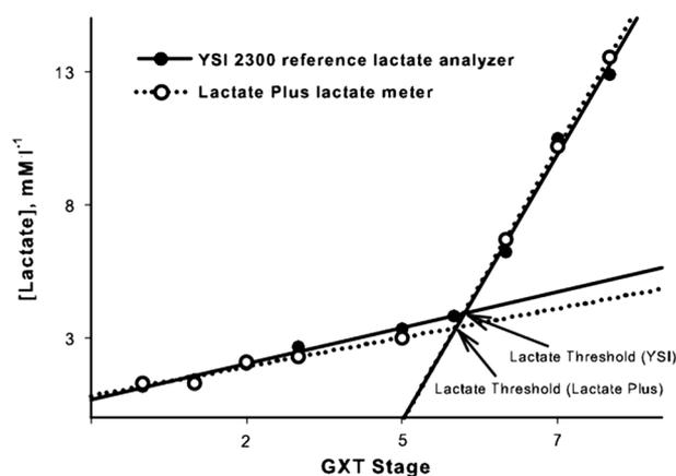
**Figure 1** Determination of the lactate threshold by visual inspection. Shown are data from a representative study participant and the lines of best fit that were determined independently for data from the YSI 2300 lactate analyzer and the Lactate Plus lactate analyzer. Blood samples could not be collected between stages 4 and 5. The Lactate Plus analyzer returned error message between stages 6 and 7.
